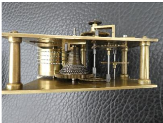
The spring and fusee mechanism of the Eberlin clock. Photograph Jim Kennett
